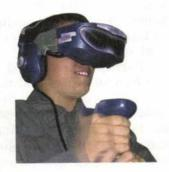
The helmet with the help of sensors picks up your eye and head movements and sends them to the computer, which changes the scene. An enemy tank fires from the south. You use the controls and your tank "moves". When the fighting is over, you know how many soldiers are "killed" and how many tanks are "destroyed". If your result isn't impressive, don't worry. You will work at warfare until you get right.
